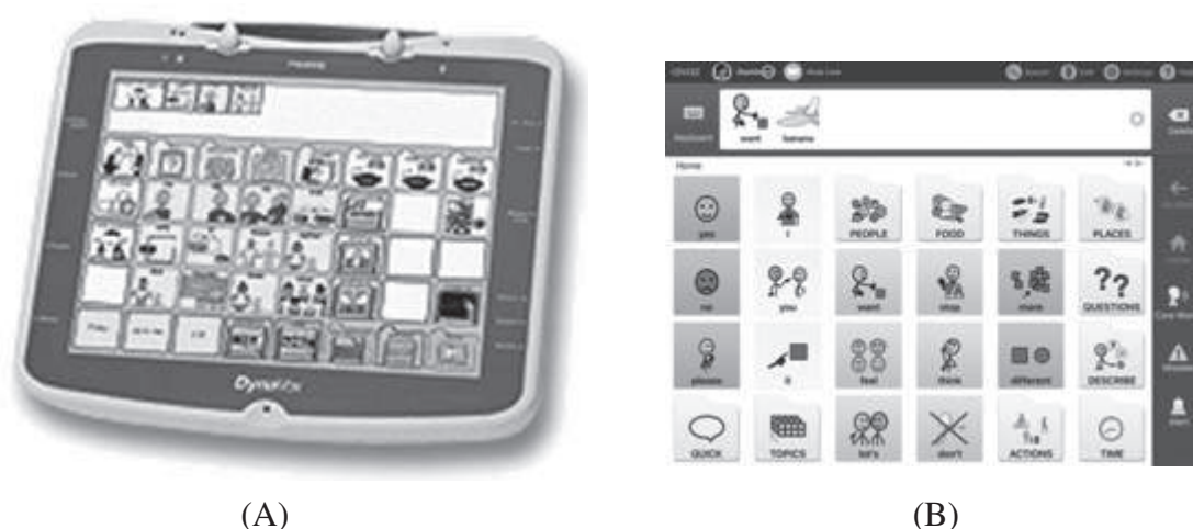
Figure 3: Examples of High Tech Device. (A) Dynavox, a touch screen based AAC device. The screen shows symbols that either play a message or change the dynamic display to display the symbols with messages to expand conversation options, and (B) Screen of Avaz AAC App
