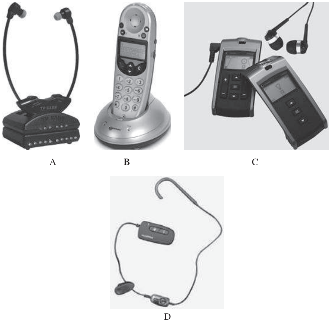
Figure 6: Examples of a few hearing assistance technologies for use by individuals with hearing impairment: (A) an infrared system for transmission and reception of auditory signals through invisible light frequencies, useful for the TV and in many live theaters and cinemas; (B) amplified cordless phone with caller ID; (C) FM system with microphones in both the transmitter and receiver for increased auditory signals, shown with earphones but also available with a neckloop that interfaces with hearing aid telecoils; (D) amplified neckloop that picks up Bluetooth signal from a cell phone and creates an induction signal for the hearing aid telecoil. (Courtesy of beyondhearingaids.com )
