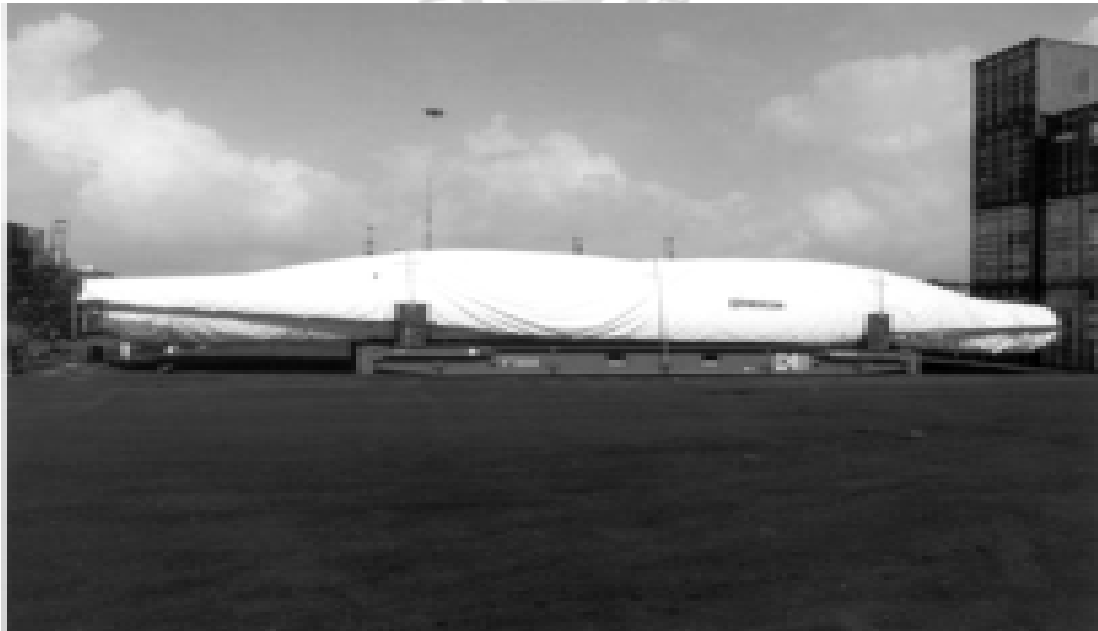
Figure 29 : A over dimensioned cargo (out-of-gauge) tied to a flat rack container
