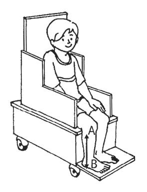
If you want to move the child around in the box seat, castors can be attached to the bottom of the seat so that it moves easily. If castors are attached, a foot rest will have to be added to the seat. To measure for the height of the foot rest, measure the child from the back of the ankle to the back of the knee (B to A).
