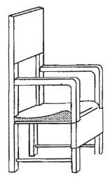
The ramp is usually two inches high at the front. It slopes gradually to cover 1/3 of the chair and becomes level with the rest of the seat. It can be made from ply wood, but should always be well padded with 1 inch thick foam which covers both the ramp and the rest of the seat.
