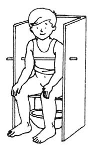
The measurements are the same as for the box seat. However the sides of the potty seat should be straight up to the shoulder. Two circular holes are made in the sides of the seat through which a rod can be inserted to ensure that the child does not fall out of the potty chair.
