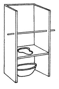
The height of the rod will be from the seat to just below the armpits. It should be at a distance of 2 inches in front of the child's chest.
