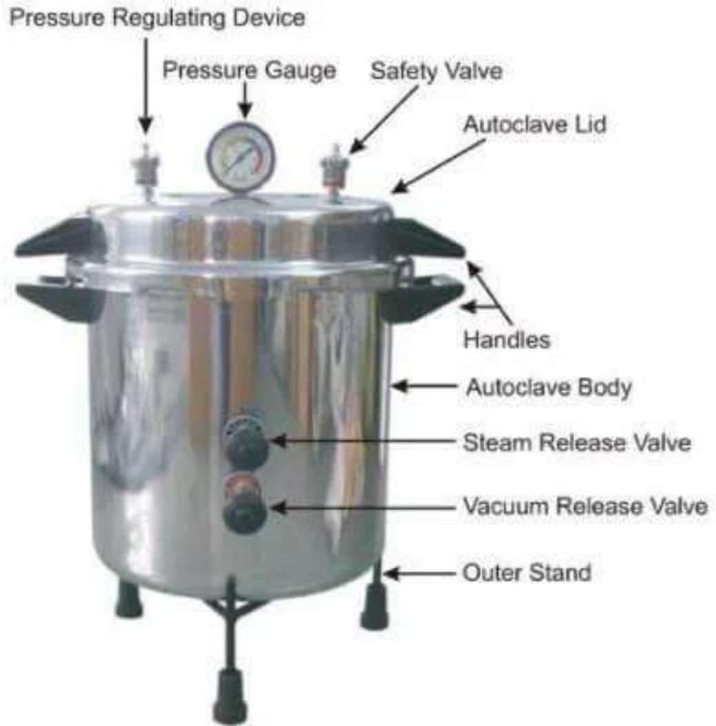
Fig 5.3 b Autoclave
